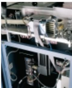
A Texas manufacturer of high-speed sorting equipment previously used a mechanical clutch-brake to drive the document infeed on one of their large sorting machines for the postal service. The mechanical clutch brake system had to be replaced sometimes in as little as every few days, incurring an
